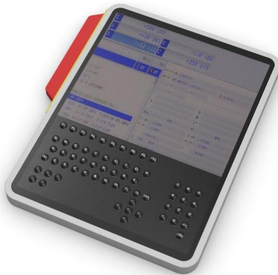
Figure 2. Touch screen with gel buttons
