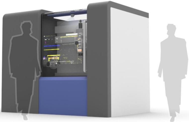
Figure 4. Projecting image on the machine tool sight window
