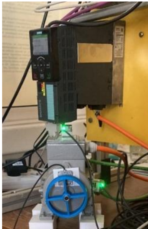
Fig. 5 Experimental setup, with electromotor and sensors
