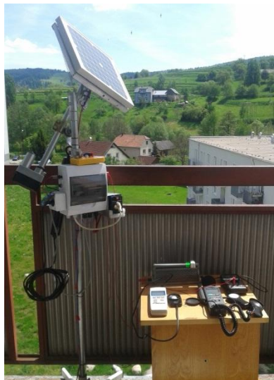
Fig. 4 Designed dual axis tracking system
