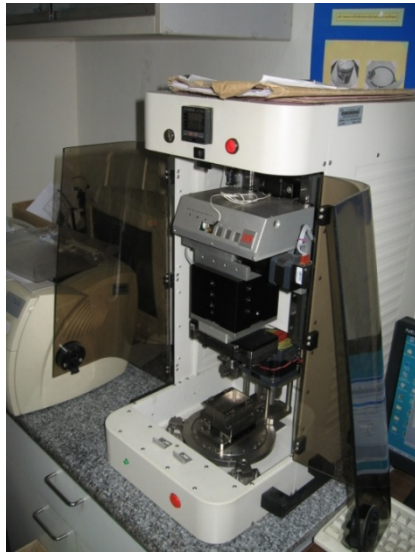
Figure 2: Micro-Tribometer testing machine (Radius of Ball Steel 6.35 mm, Applied Load 200 N, Stroke 10 mm, Oscillates Frequency 10 Hz, Duration time 33 min 20 sec (400m), Temperature 85\pm 3 °C, Humidity 40-60%)
