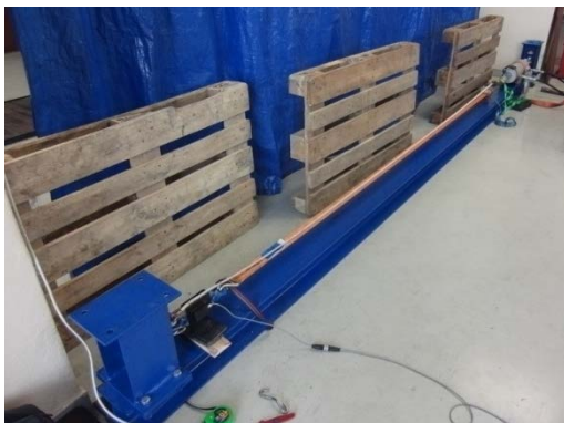
Fig. 2 Testing stand to test tension forces in lashing straps and measuring distances for strap samples
