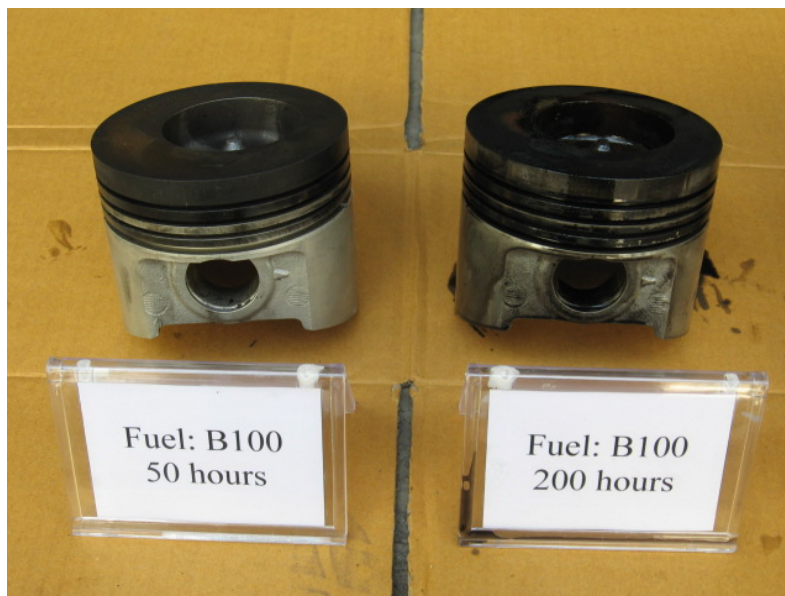
Figure 4: Piston heads after each engine test
