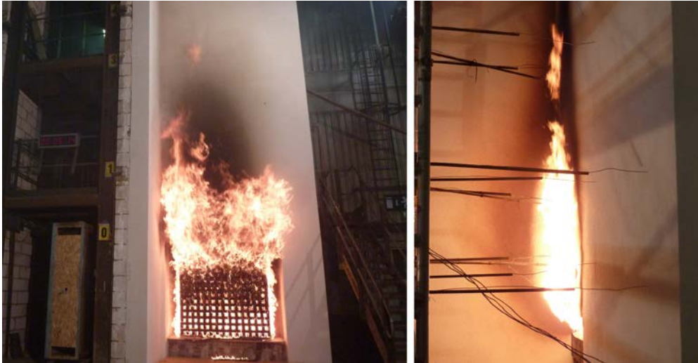
Figure 1: Except straining of heading, there was another breach of ETICS render ca. 1,0 m above fire source. Left: BS 8414-1 [2], right: DIN 4102-20 [3]. Author: M. Smolka
