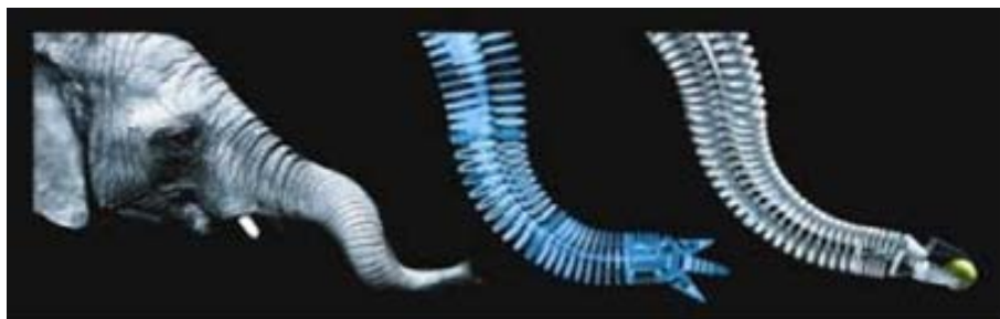
Fig. 1 Elephant trunk and hyper-redundant mechanism from Festo
